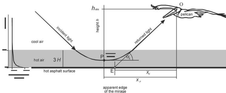
**Fig. 1.** Schematic tracing of the ray of light taking part in the formation of the apparent edge  $E$  of a mirage above a horizontal hot asphalt surface viewed by a brown pelican gliding with eyes at height  $h_{\text{obs}}$ . The exponential decrease of the air temperature  $T(h,H)$  from  $T_{\text{max}}$  to  $T_{\text{min}}$  with increasing height  $h$  is shown in the left inset, where  $H$  is the characteristic height of the temperature profile above the asphalt surface
