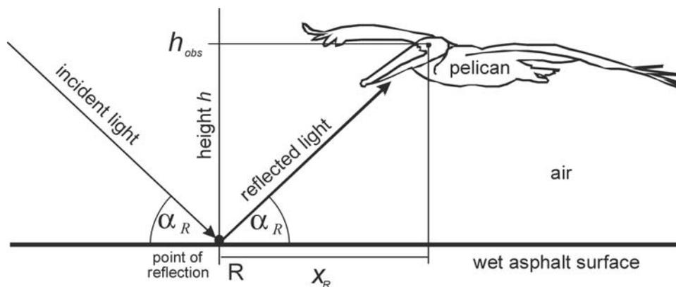
**Fig. 3.** Schematic tracing of a ray of light reflected from a horizontal, wet asphalt surface viewed by a brown pelican (*Pelecanus occidentalis*) gliding with eyes at height  $h_{\text{obs}}$ . Pelicans often glide effortlessly only about 50–60 cm off the water surface. Then their head is carried over the shoulders with the neck in a vertical S-curve
