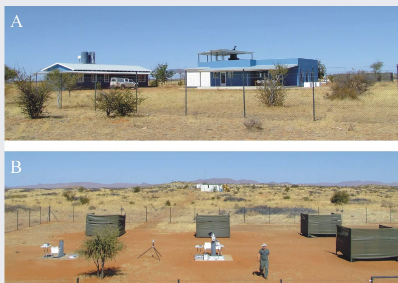
Figure 2: The two buildings of the Isabis Astrofarm (A) and the area behind them with 8 telescope stands, of which only 6 are visible in the picture (B). The nearer central stand is already equipped with the team's polarisation telescope. The two white buildings in the distance belong to the Russian space debris monitoring station under construction (photos by Gábor Horváth).
